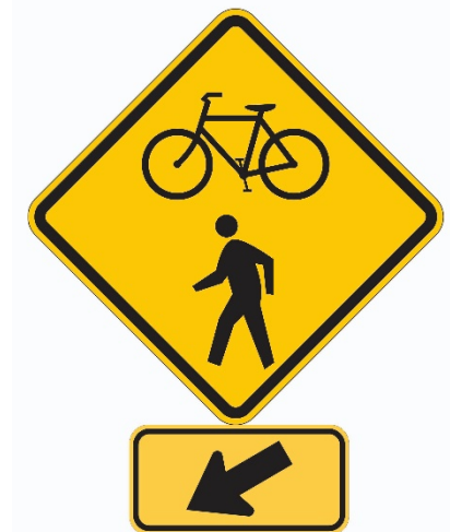
Figure 3-13: An example of a Trail Crossing Warning Sign
