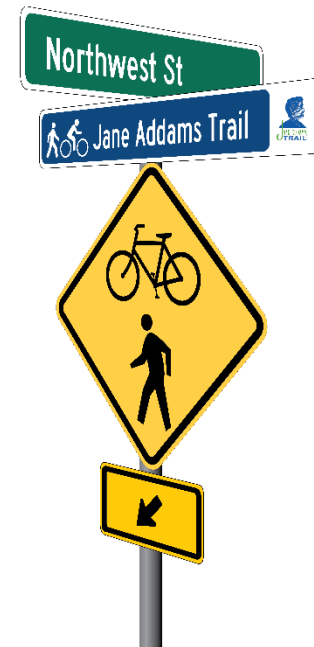
Figure 3-12: A Street Name/Trail Name Sign placed above a Crossing Warning Sign
